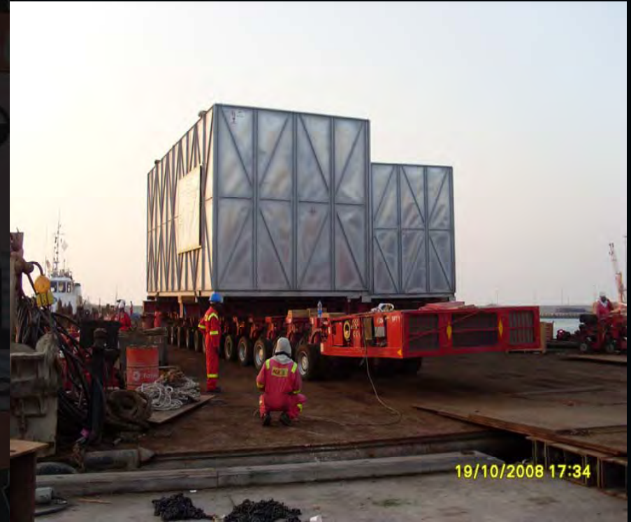
2 x 90 Ton Compressors being loaded onto barge at Abu Dhabi Port for onward movement to Mussafah for Habshan OAG III Project
