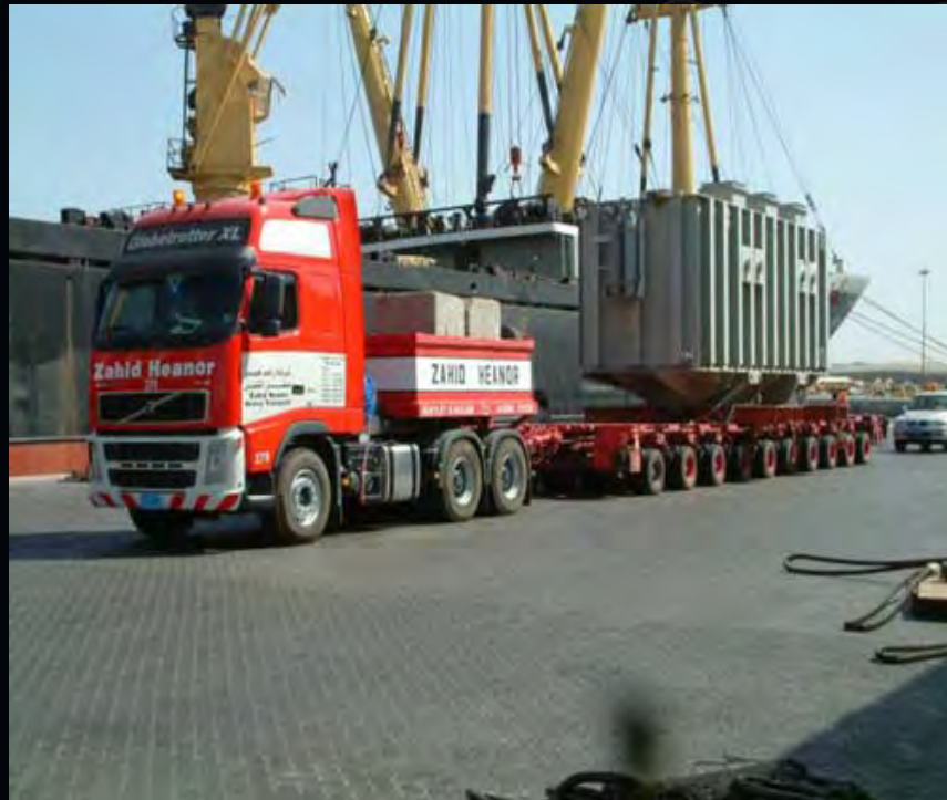
180 Ton transformer being brought along side vessel at Jebel Ali, Dubai
