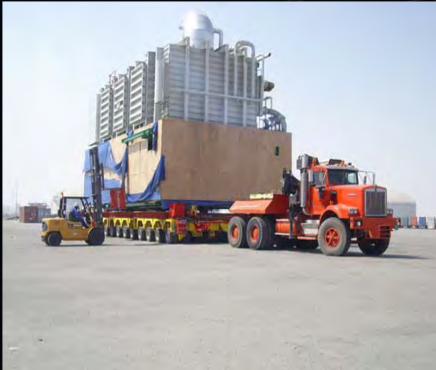
140 Ton Evaporator being moved from Messaied Port - Qatar
