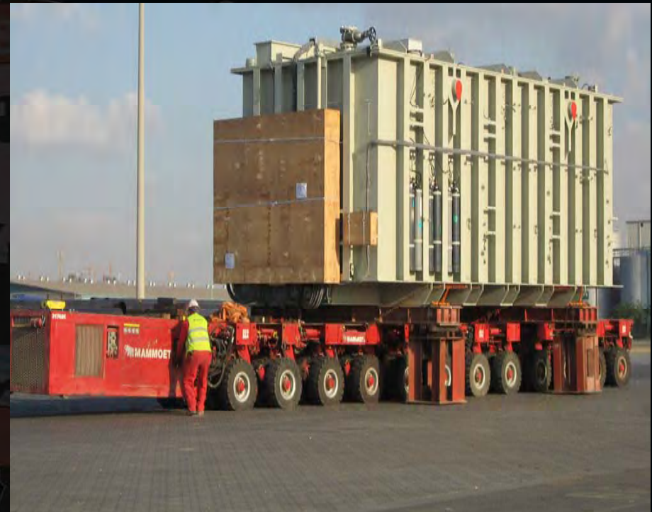
250 Ton Transformer being received on hydraulic trailer at Jebel Ali, Dubai
